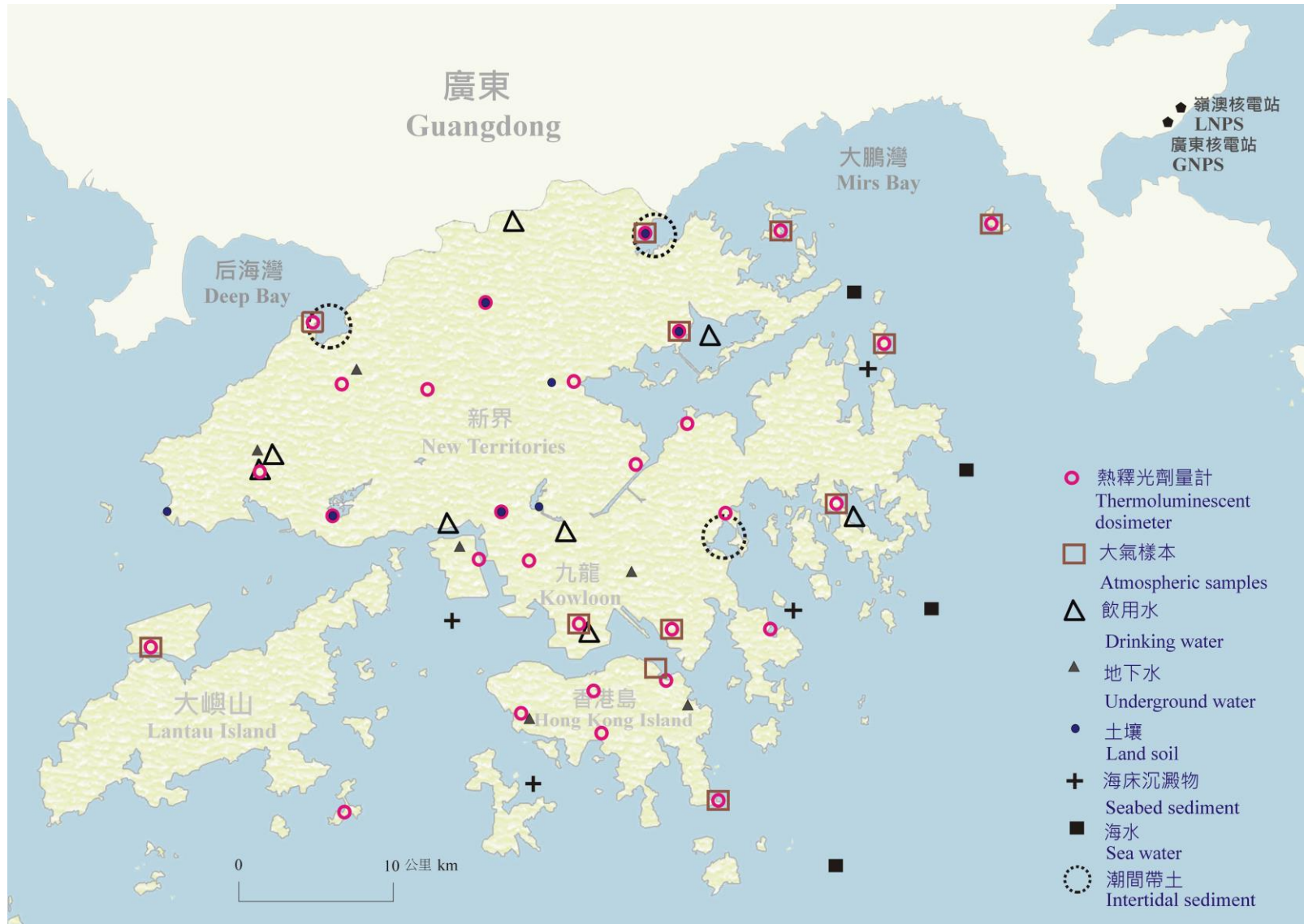
圖 2. 熱釋光劑量計網絡及二零一六年環境樣本收集點。 Figure 2. Thermoluminescent dosimeter network and locations for collection of environmental samples in 2016.
