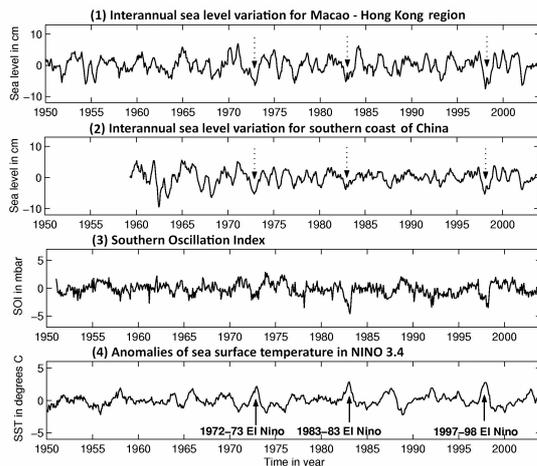
Figure 2 - Effects of ENSO on the mean sea-levels over coast of southern China (Ding et al 2004).
