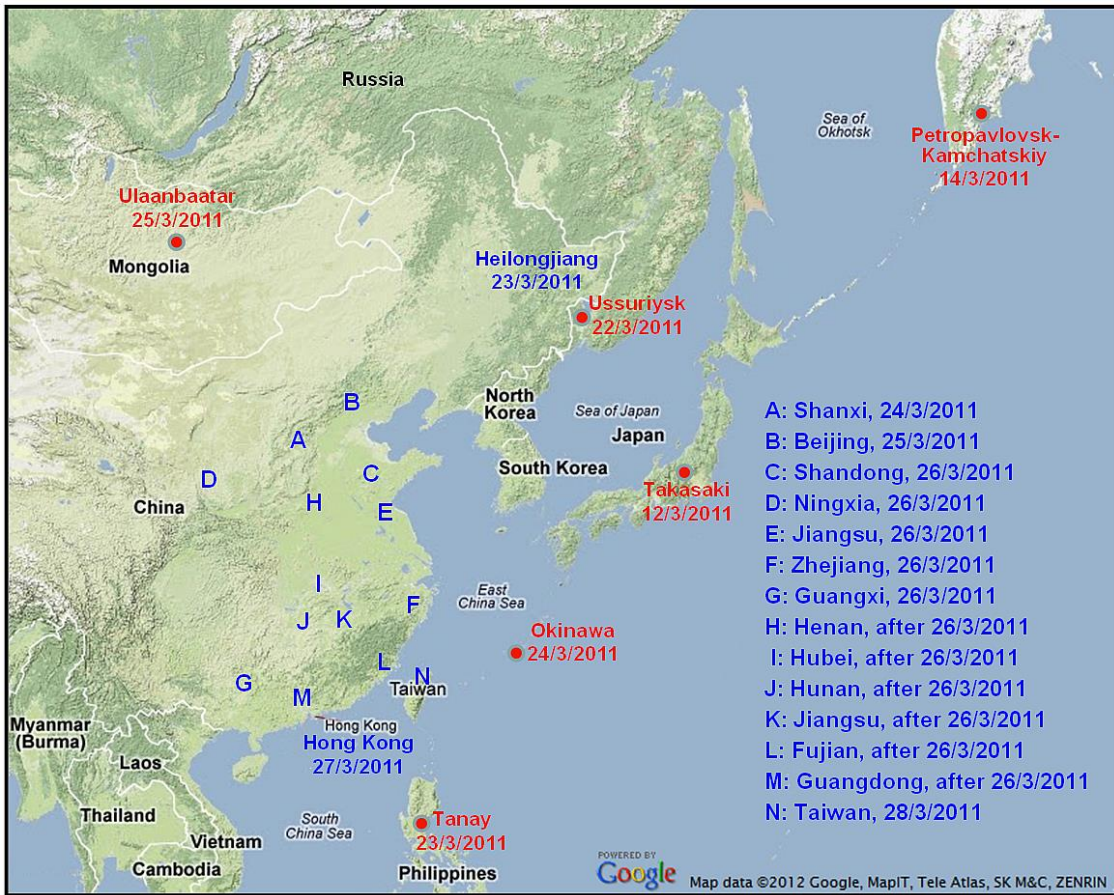
Figure 8 Dates of first detection of ^{131}\text{I} from airborne particulates originating from the Fukushima nuclear accident as detected in various places over Asia. CTBTO monitoring stations are marked with red dots, while those operated by local authorities are marked in blue. The sampling period for monitoring stations in mainland China and Hong Kong was 24 hours, while that in Taiwan was a 7-day period from 22 to 28 March. (Sources: CTBTO; Radiation Monitoring Technical Centre, Hangzhou; and Taiwan Atomic Energy Council)
