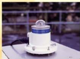
Figure 1 The Hong Kong Observatory's "broadband" UV meter at the King's Park Meteorological Station
