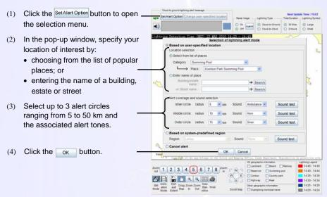
The lightning alert webpage will be updated automatically. When lightning is detected within the specified ranges, users will be alerted with alert message and sound through their computer or mobile phone.
