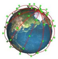
In the Iridium network, each satellite communicates with other nearby satellites in front, behind and in adjacent orbits. Data messages can be routed anywhere in the world by the network. Calls can be made from a data unit on the ground to a satellite above it. That satellite then transfers the information to another satellite and then down to a ground receiving station for relaying the call to the recipient.
