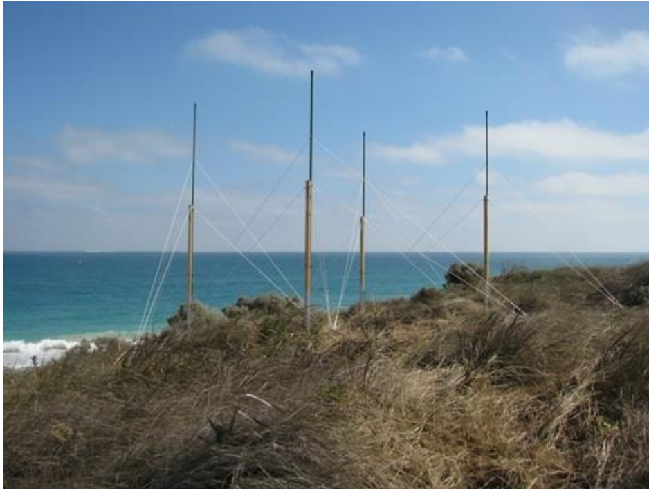
Figure 2 An array of antennas for the HF ocean radars in western Australia, part of the Australian Integrated Marine Observing System/Australian Coastal Ocean Radar Network. (Photo courtesy of Professor Malcolm Heron, James Cook University, Townsville, Australia)
