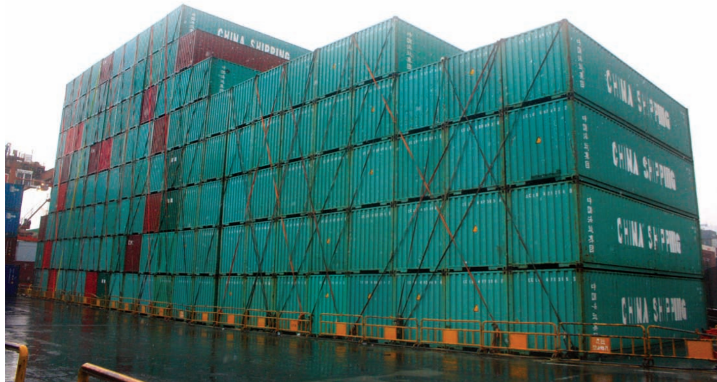
Containers lashed in readiness for adverse weather conditions
