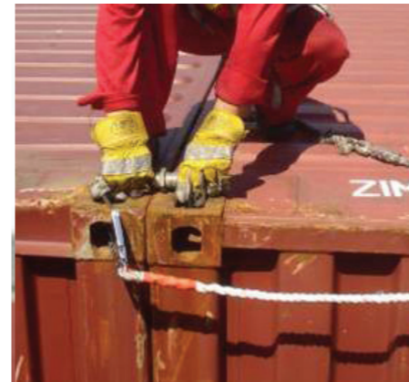
Bridge fitting prevents movement between containers
