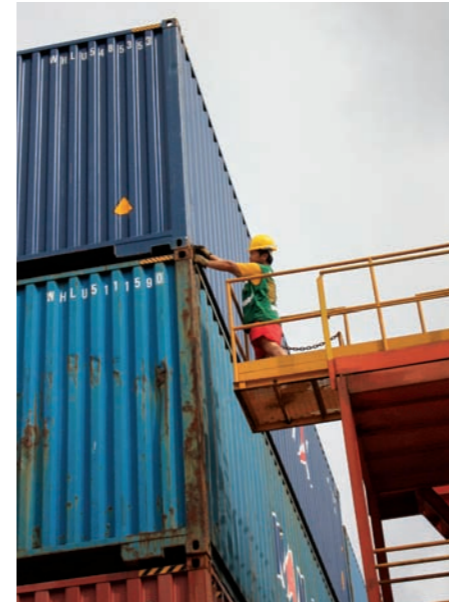
Worker securing a container
