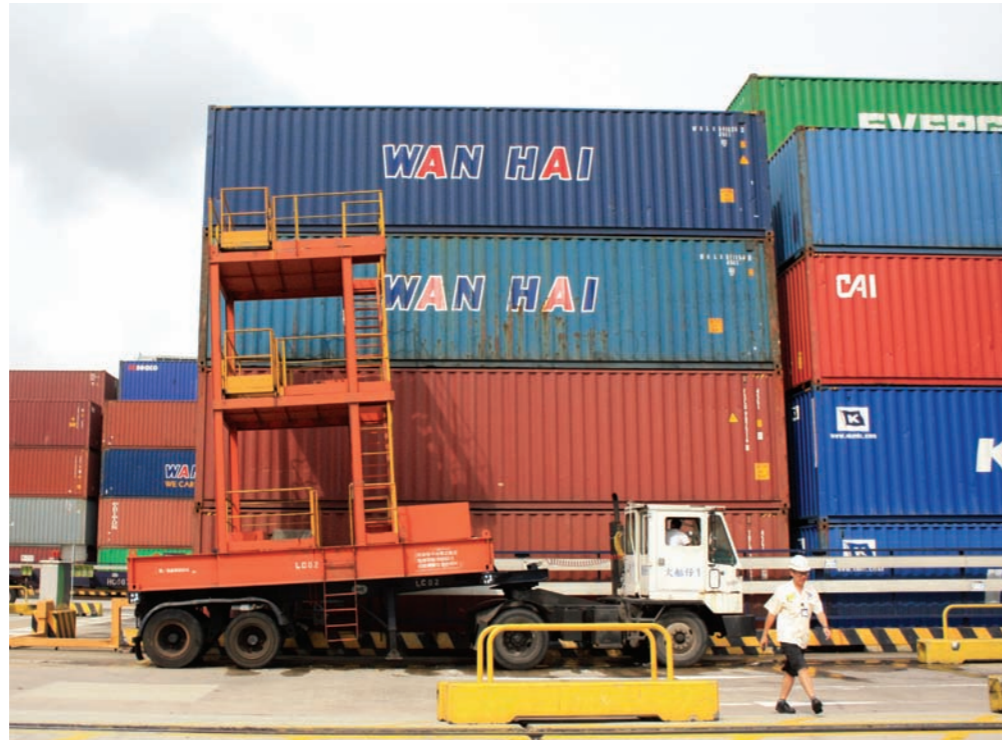
A multi-level scaffold platform, also known as a "wooden horse", ready for container lashing
