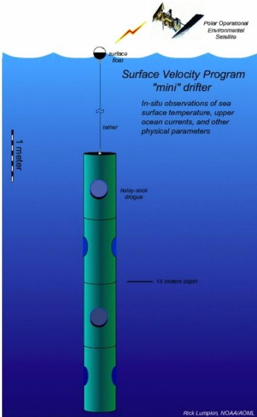
Schematic diagram of a drifter buoy at sea. (Courtesy of R. Lumpkin and P. Mayra of AOML, NOAA)
