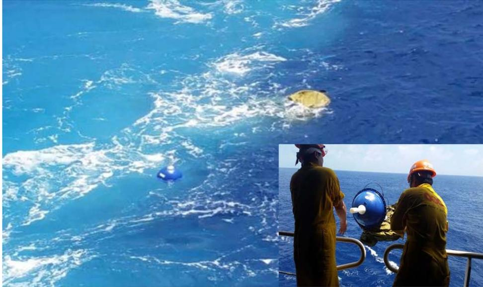
Deployment of a drifter buoy by crew members on board an ocean-going vessel.
