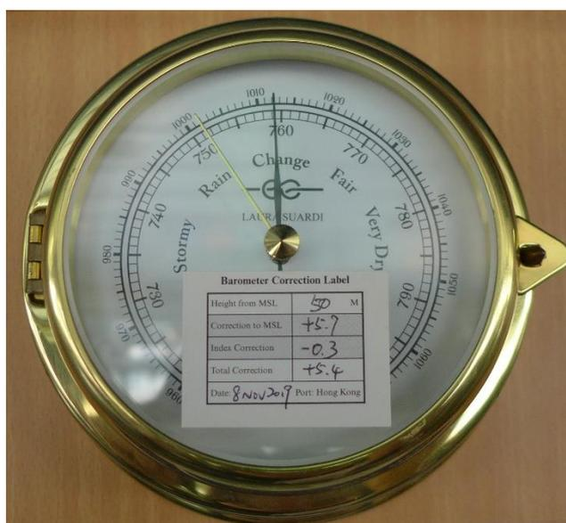
Figure 2. Aneroid barometer
