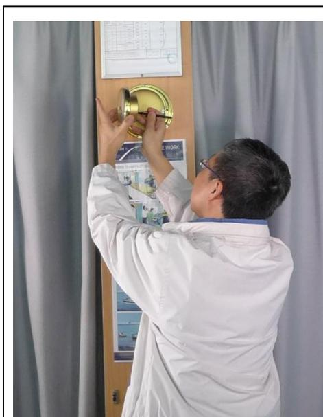
Figure 1. Barometer calibration by Port Meteorological Officer
