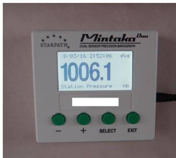
Figure 4. High precision digital barometer for mariners
