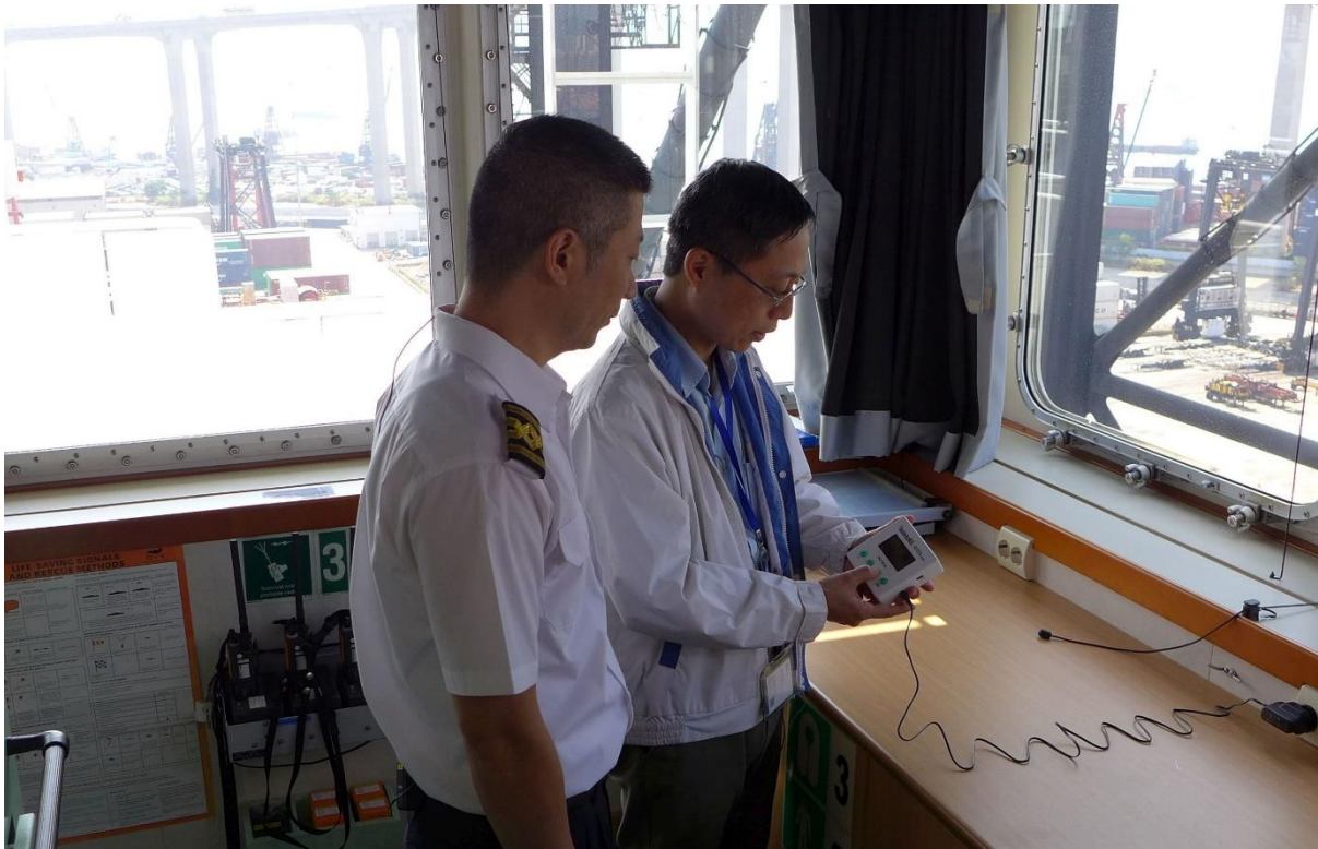
Port Meteorological Officer demonstrating to the Captain of a newly recruited HKVOS on the operation of a digital barograph
