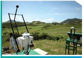
Picture shows the direct and diffuse solar radiation instruments (left in Kau Sai Chau solar station mounted on a sun tracker and the global solar radiation sensor (right).
