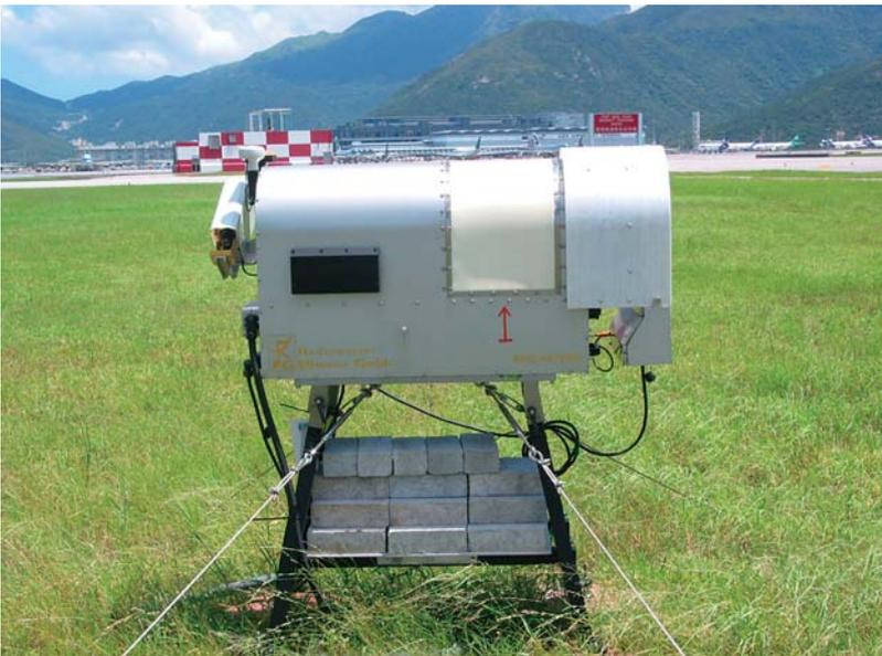
Figure 1: The microwave radiometer operating at the airport.
