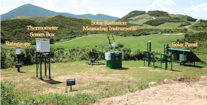
Meteorological instruments at the Kau Sai Chau Solar Radiation Station
