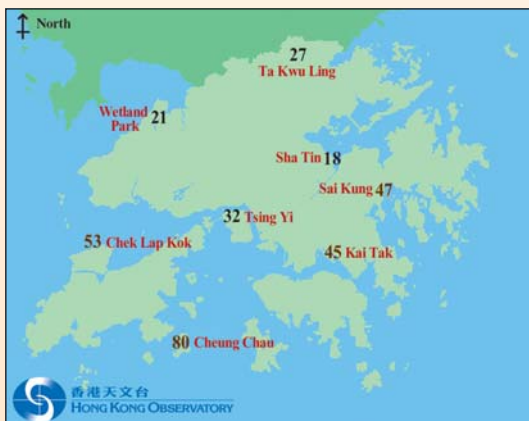
Figure 1 : The maximum wind speeds recorded at the eight reference wind stations from 3:41 p.m. to 4:40 p.m. on 19 April. Among them, Chek Lap Kok, Cheung Chau, Kai Tak and Sai Kung recorded strong or higher wind strength. (Wind speed in kilometre/hour)
