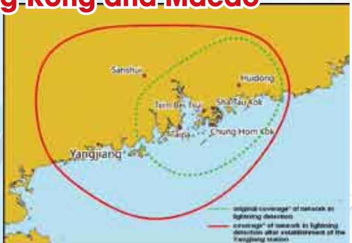
▲ Significant increase in spatial coverage of the Lightning Location Network.
