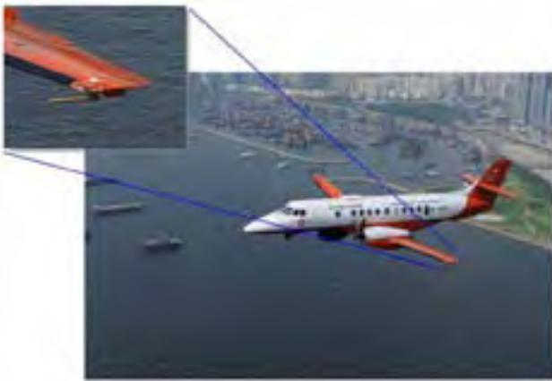
Figure 1: A GFS fixed wing aircraft with a data probe mounted on the wing tip collects meteorological data in the vicinity of the HKIA regularly
