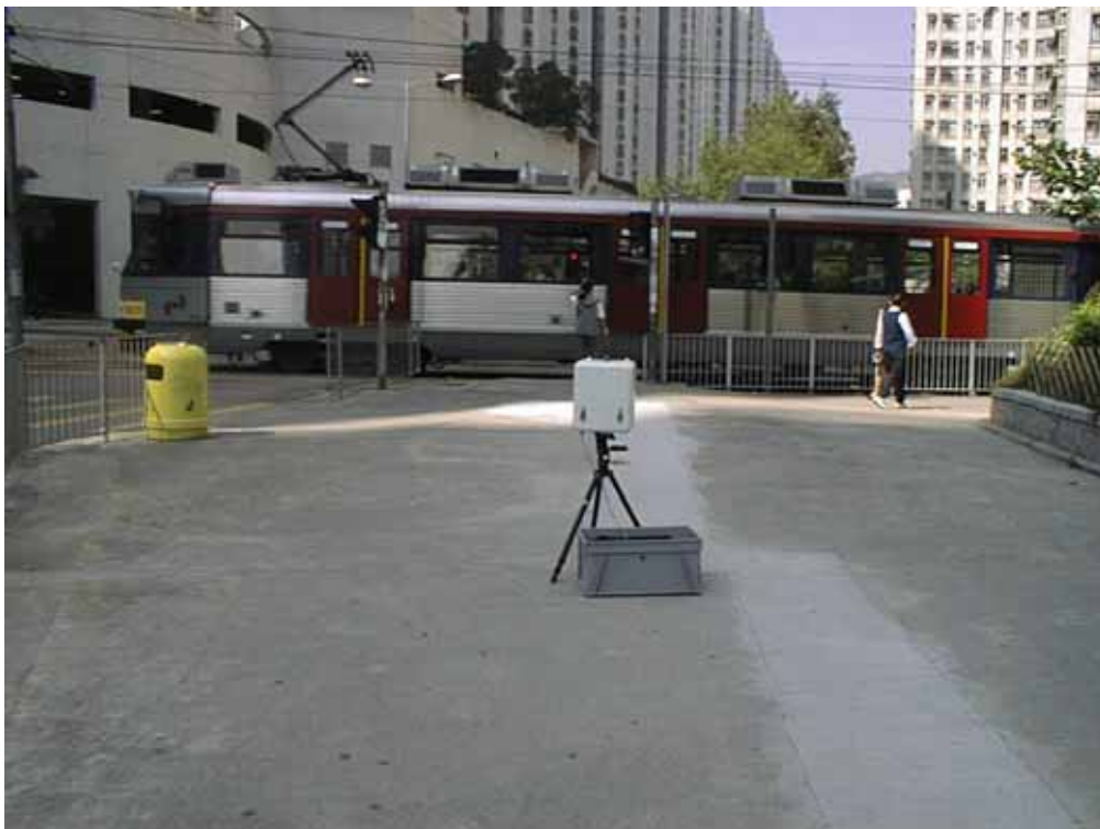
Figure 3 Measurement of the gamma absorbed dose rate in air at street level at Tuen Mun, New Territories
