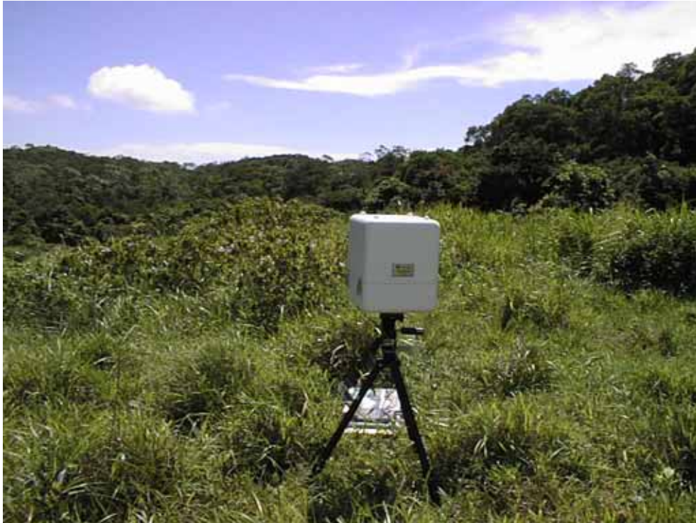
Figure 2 Measurement of the gamma absorbed dose rate in air in an open field at Ngong Ping, Lantau
