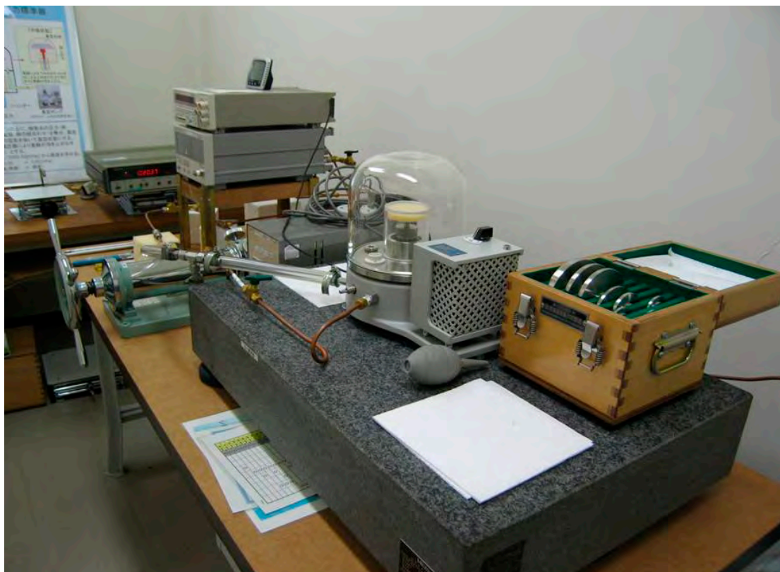
Figure 2 The Japan Meteorological Agency Primary Standard Barometer
