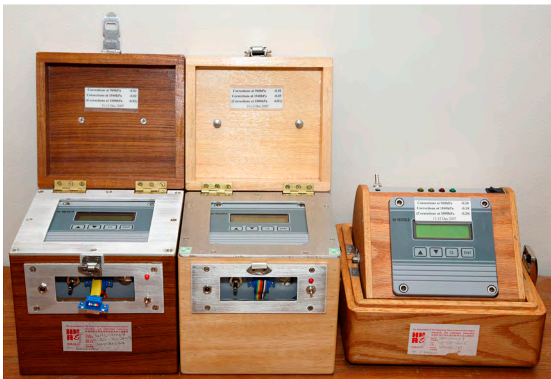
Figure 3 Travelling Standard Precision Digital Barometers
