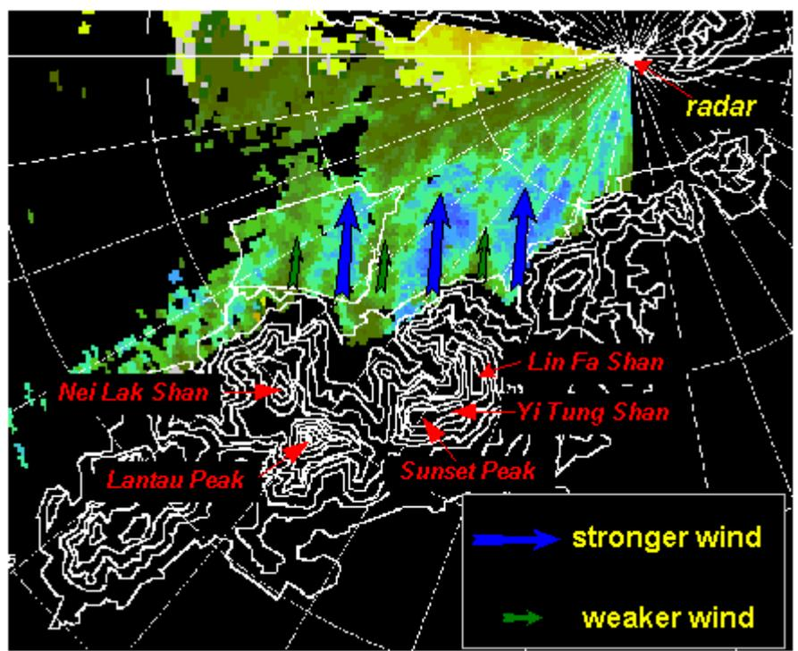
Figure 2 Radar picture of radial winds at 0.6° elevation angle at 02:56 H on 8 June 1999.
