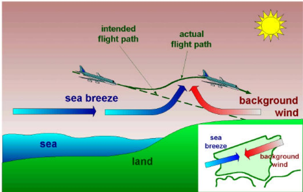
Figure 7 Effect of a sea breeze on an approaching aircraft.
