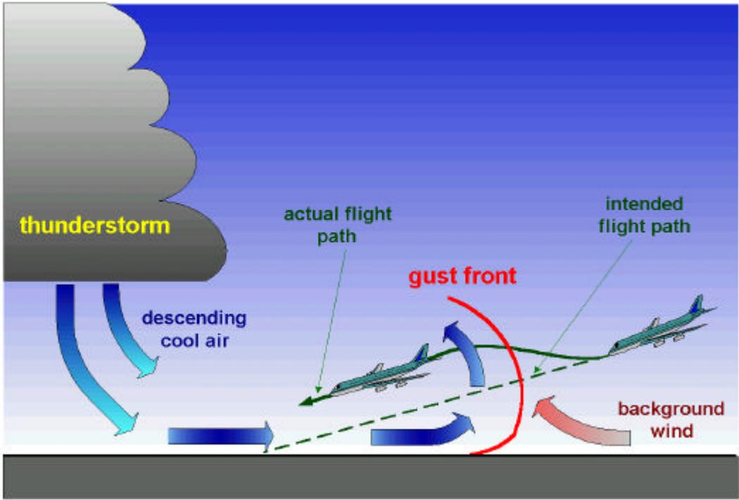
Figure 4 Effect of a gust front on an approaching aircraft.
