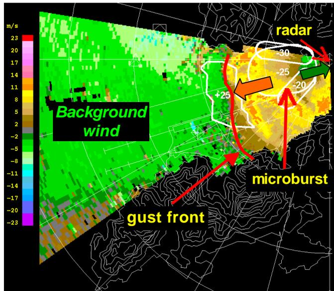
Figure 6 Radar picture of radial winds at  $0.6^\circ$  elevation angle at 15:37 H on 3 September 1999.
