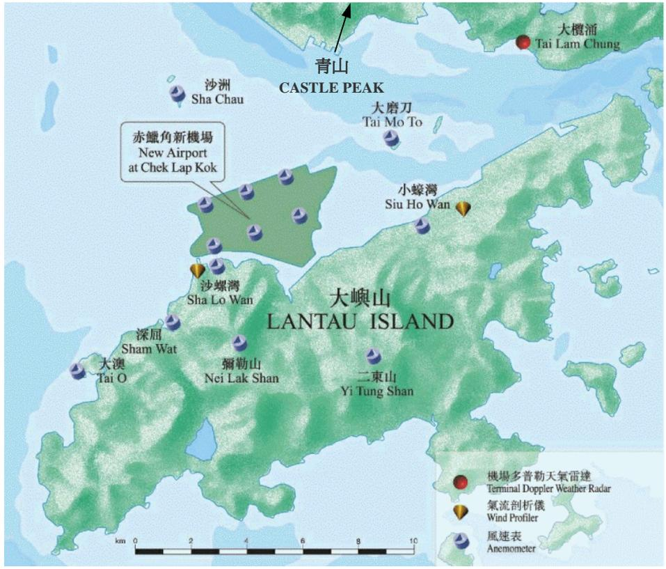
Figure 1 Location of weather sensors in support of the windshear and turbulence alerting service.
