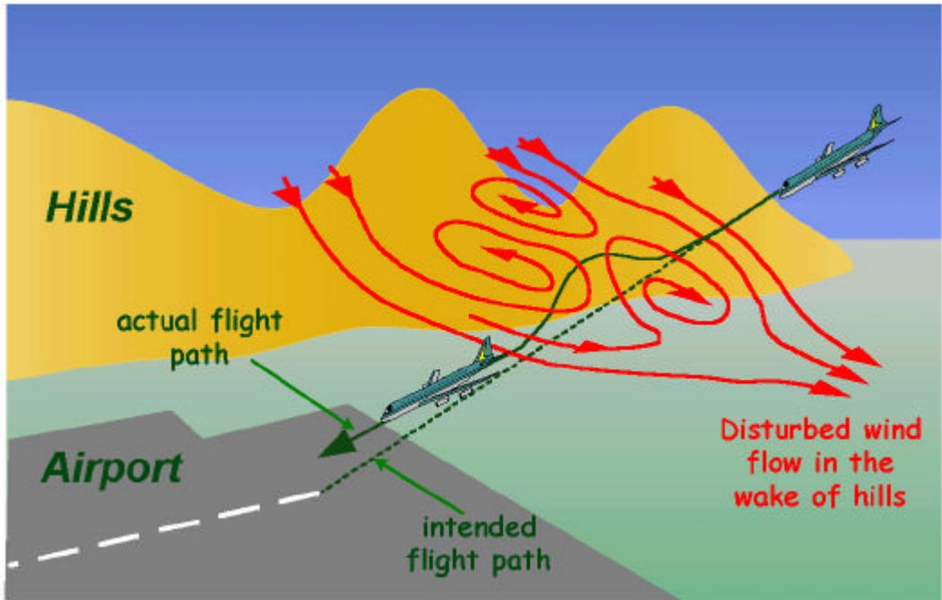
Figure 3 Disturbed wind flow in the wake of hills, as simulated by a computer model.
