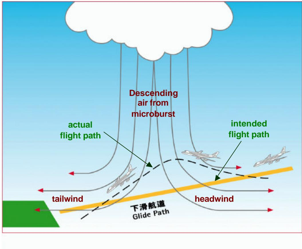
Figure 5 Effect of a microburst on an approaching aircraft.
