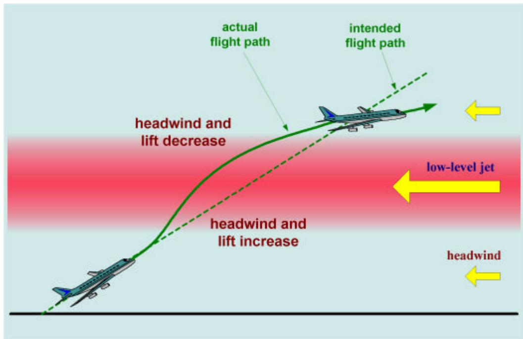
Figure 8 Effect of a low-level jet on a departing aircraft.
