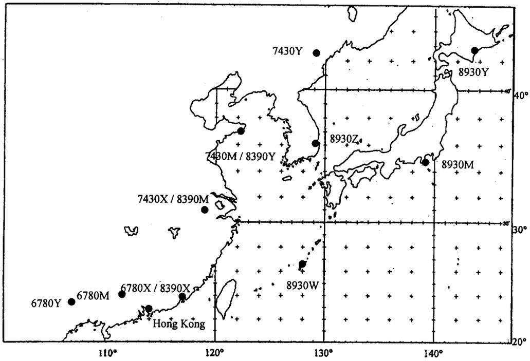
Figure 3. Locations of LORAN-C Chains
