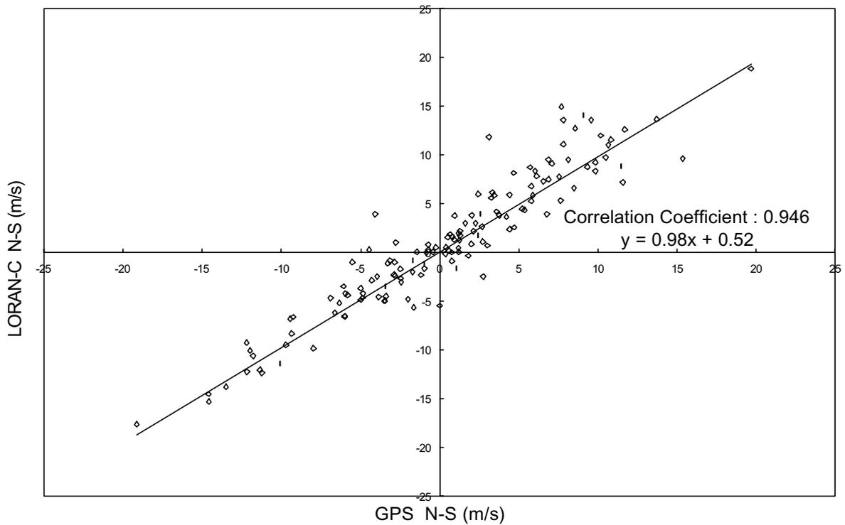
Figure 2. Scatter Diagram of the North-South Components Measured by the LORAN-C and GPS Wind-finding Systems
