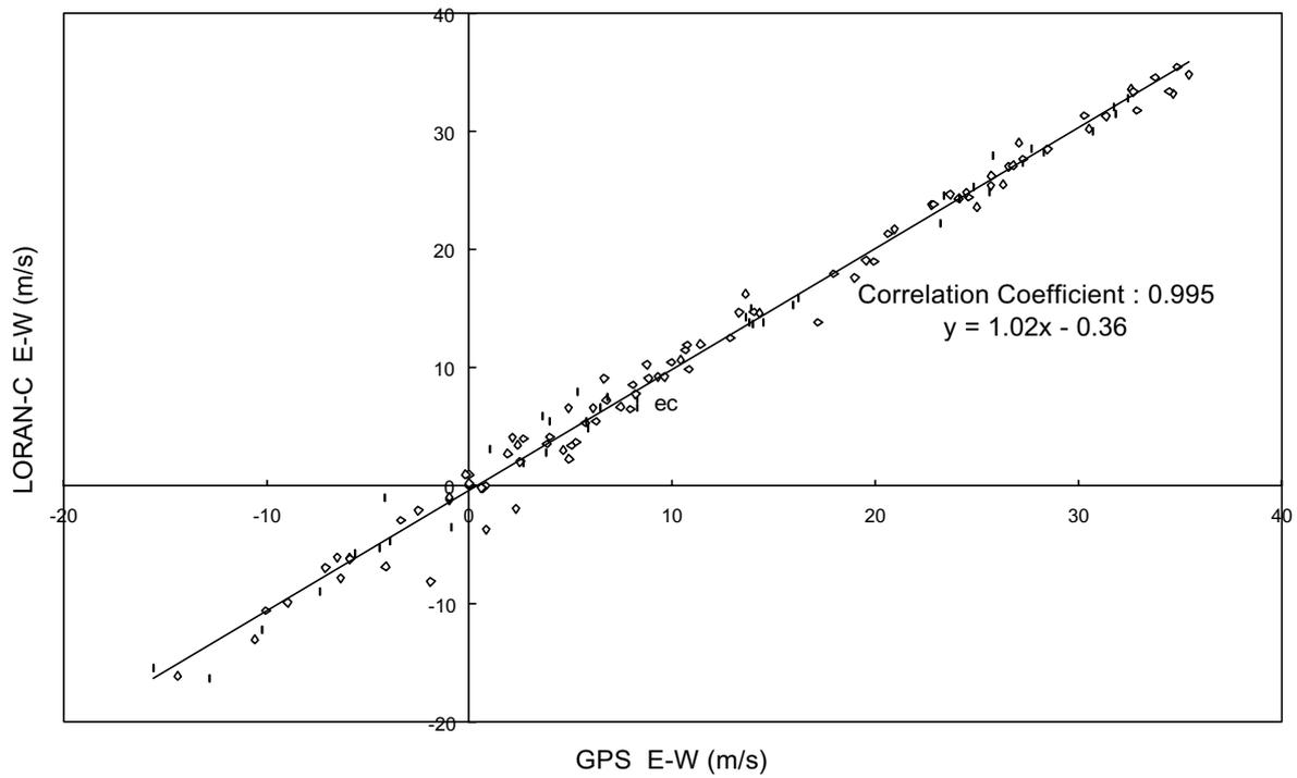
Figure 1. Scatter Diagram of the East-West Components Measured by the LORAN-C and GPS Wind-finding Systems
