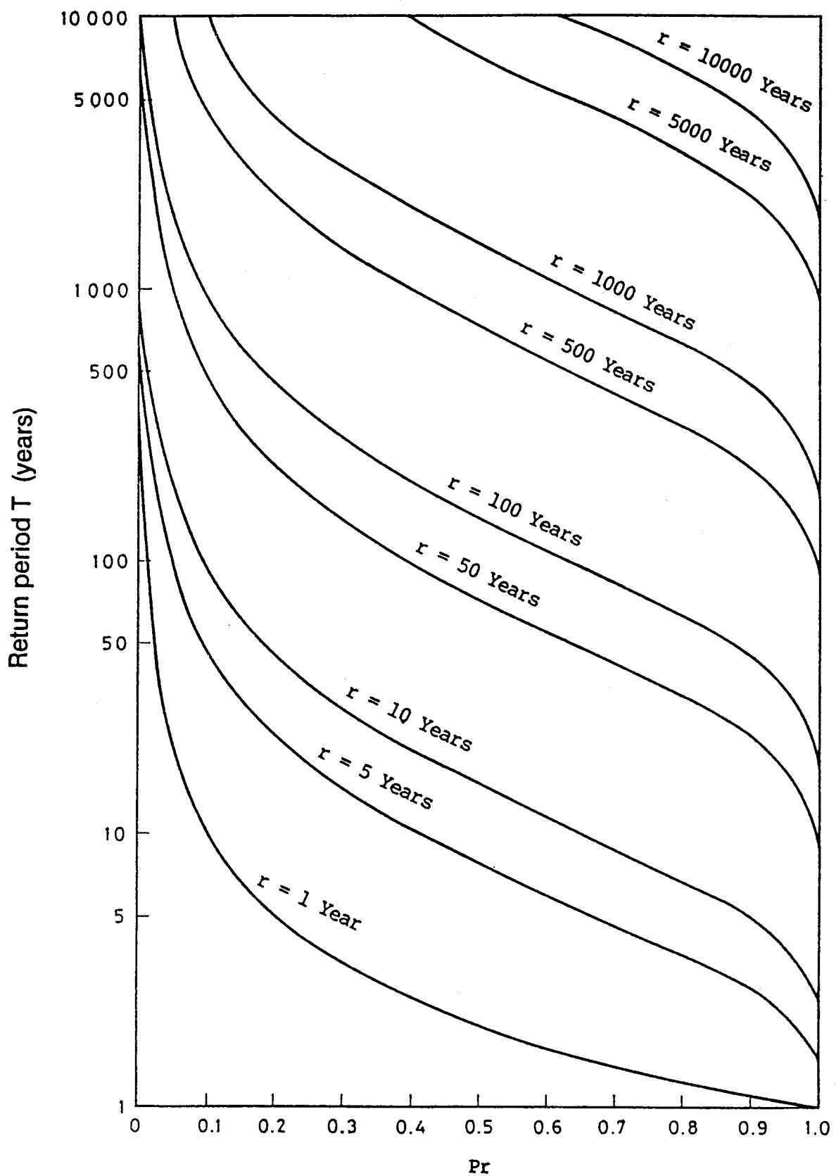
Fig. 18 The probability that a level with a return period  $T$  will be reached or exceeded at least once in a period  $r$
