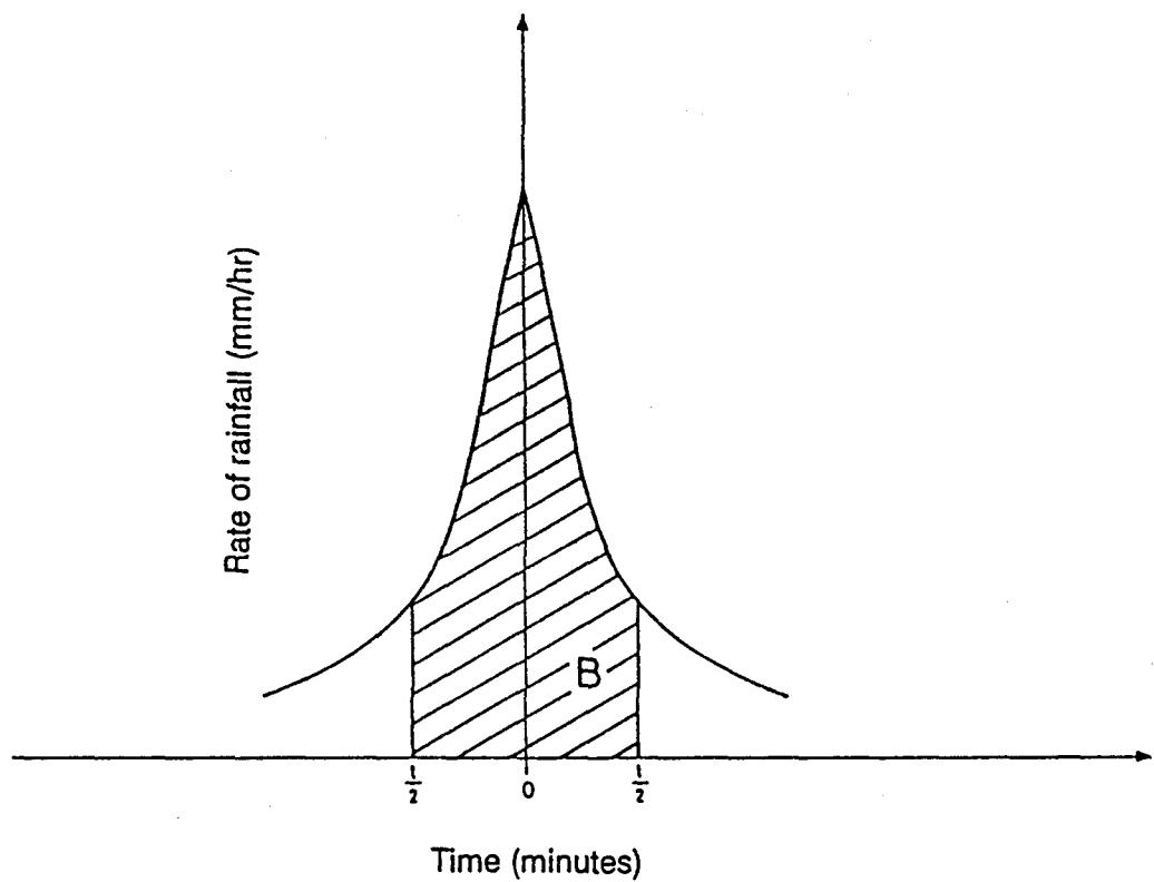
Fig. 12 A schematic diagram showing a design storm profile corresponding to the same return period as in Fig. 11 with the constraint of having shaded area A = area B for any value of t
