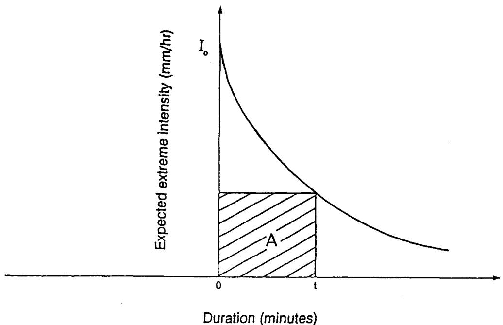
Fig. 11 A typical plot of expected extreme intensity versus duration for a given return period
