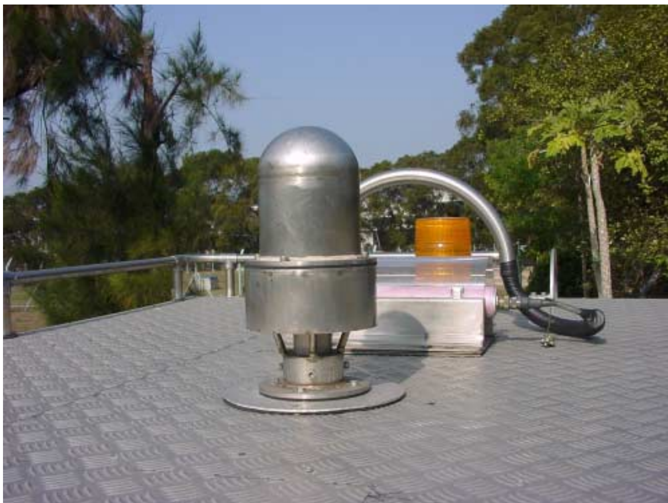
Figure 6 Air inlet of the air samplers mounted on the rooftop of the Mobile Radiation Monitoring Station
