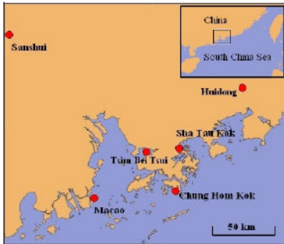
Figure 9 Distribution of sensors in the HKO lightning location network. The rectangle in the inset map shows the location and coverage of the main map (from Lee, 2009).
