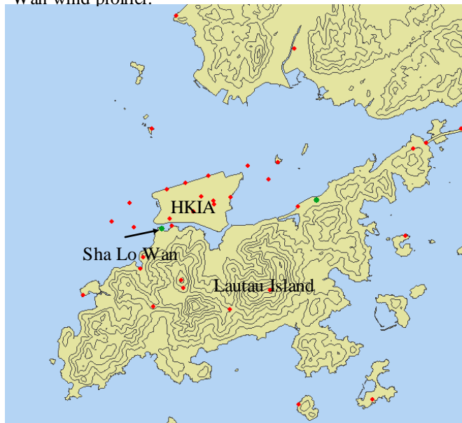
Figure 1 The geographical setup around HKIA. Height contours are in 100 m. The red dots are the locations of the surface anemometers, whereas the green dots are the wind profilers.
