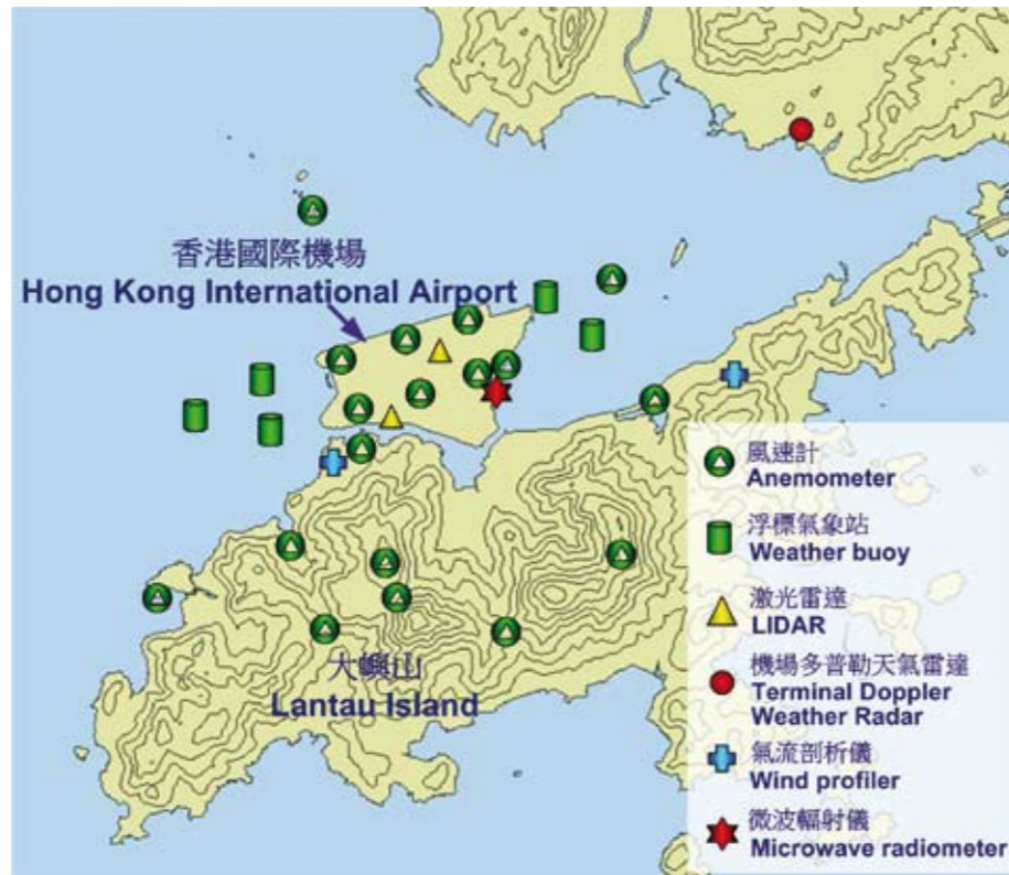
FIGURE 1: A map showing the many meteorological instruments installed inside and around HKIA for the monitoring of low-level windshear
