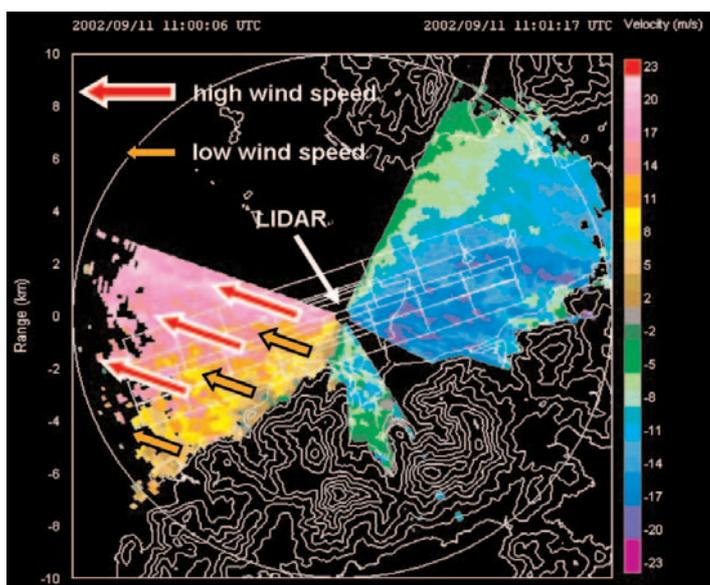
Figure 5 — LIDAR Doppler radial velocity pattern from a 1.0° elevation scan, revealing the presence of high- and low-speed streaks downwind of rugged terrain
