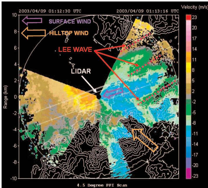
Figure 6 — LIDAR Doppler radial velocity pattern from a 4.5° elevation scan, revealing the presence of a lee-wave pattern to the east of the airport. An aircraft departing towards the east a few minutes later reported a loss of 15 knots at a height of about 520 m.
