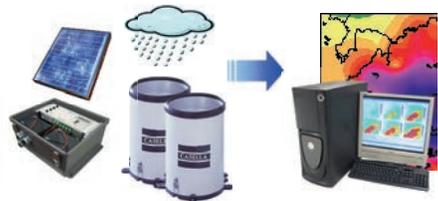
*Figure 4: Real-time rainfall data is transmitted to GEO and HKO for use in the Landslip Warning System*
