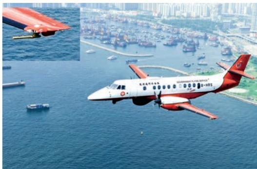
*GFS Jetstream 41 aircraft with a specially designed data collection probe.*
