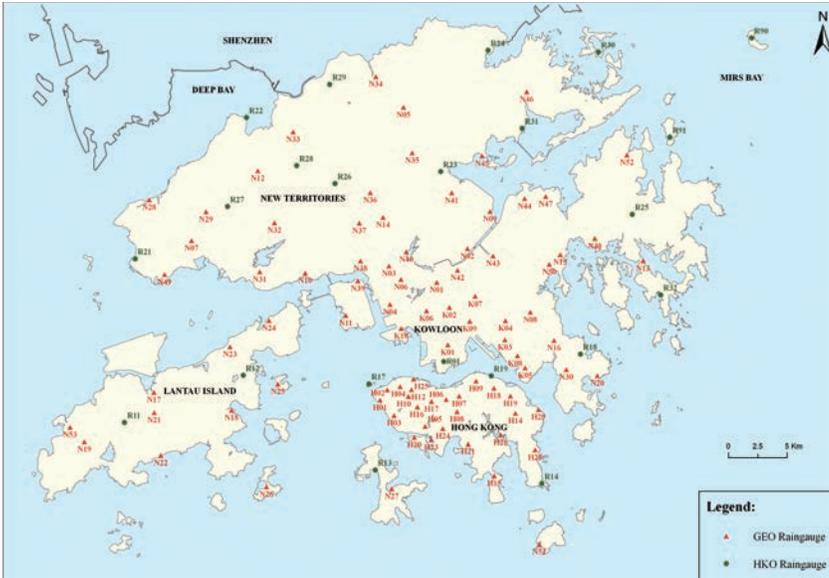
*Figure 5: Locations of GEO rain gauges and HKO rain gauges in Hong Kong*
