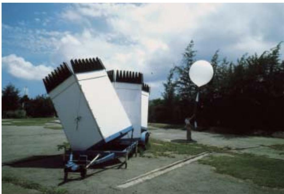
Fig. 4.29 The Doppler acoustic radar system used by the Observatory to measure wind speed and wind directions (1983). Courtesy Hong Kong SAR Information Services Department
