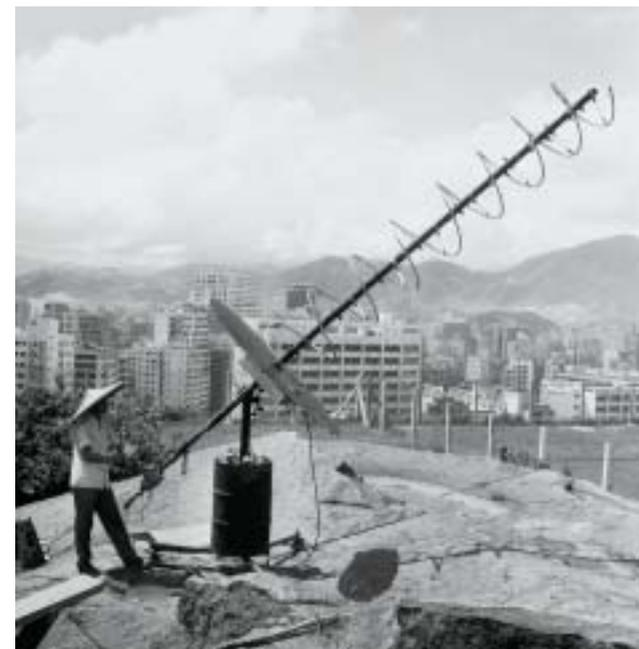
Fig. 4.30 Observatory staff manually aligning an aerial to receive images from a US weather satellite, at a home-made tracker station. (1965). Courtesy Hong Kong SAR Public Records Office
