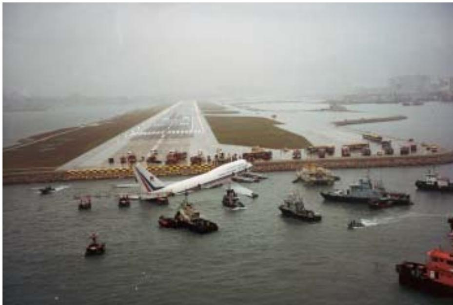
Fig. 4.18 Situated in the centre of the city, Kai Tak International Airport had its runway built into the sea, making it prone to accidents during adverse weather conditions. In 1993, an aircraft overshoot the runway and ploughed into the harbour. Courtesy Hong Kong SAR Information Services Department
