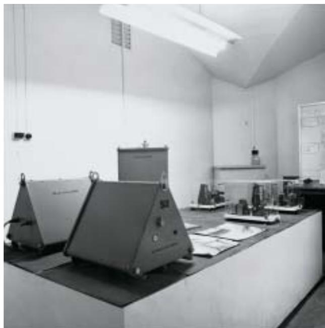
Fig. 3.43 Seismographs housed inside the double-walled cellar. Courtesy Hong Kong SAR Information Services Department
