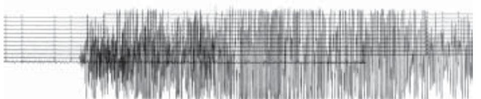
Fig. 3.45 A seismogram recording an earthquake in Taiwan of magnitude 6.5 on the Richter Scale on 16 September 1994. Courtesy Hong Kong Observatory
