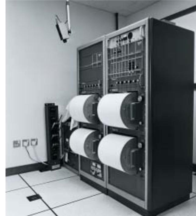
Fig. 3.44 Seismographs housed inside the Observatory's seismological laboratory. Courtesy Hong Kong SAR Information Services Department
