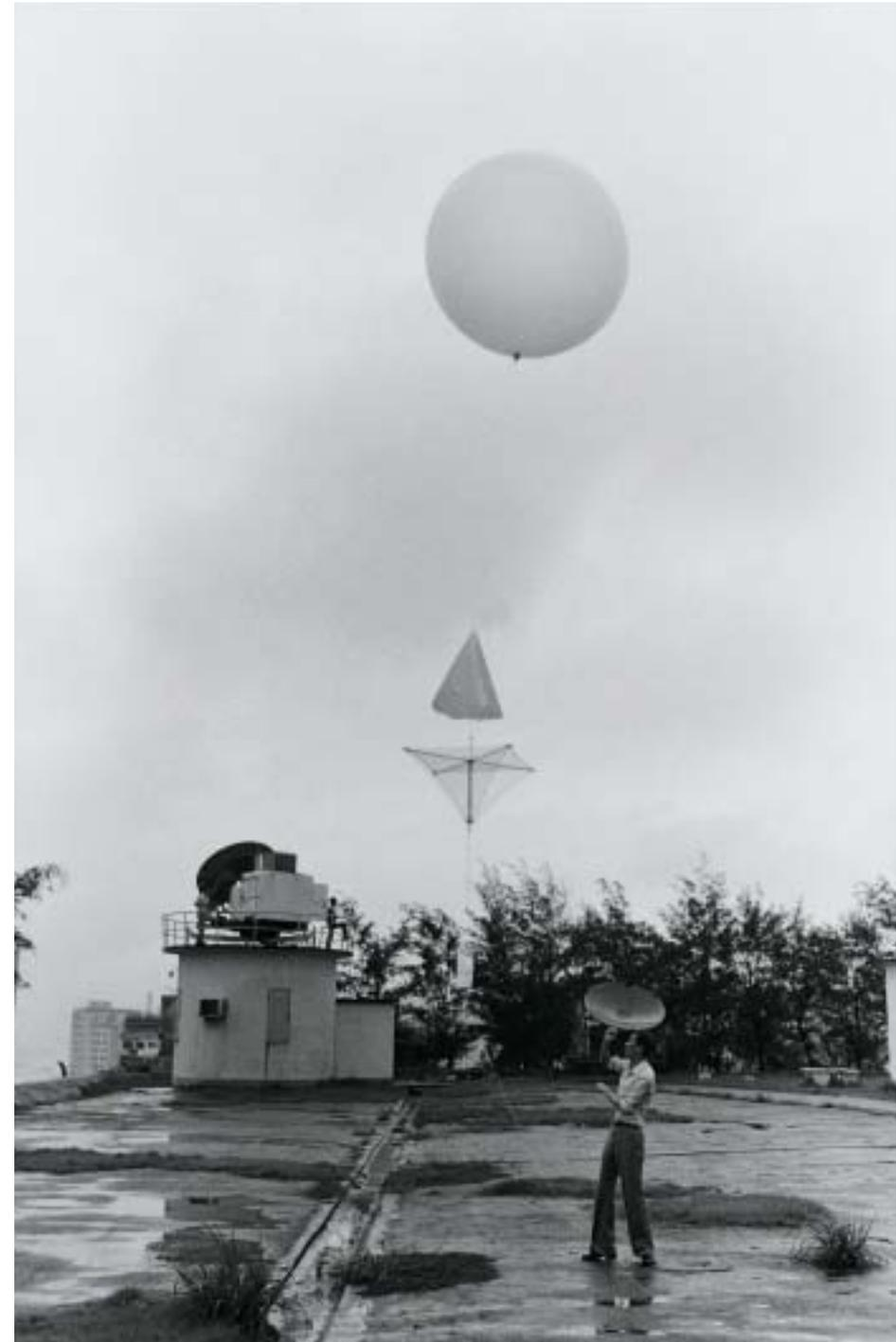
*Fig. 3.40* A sounding balloon sent out with wireless meteorological instruments. Photograph taken on 5 June 1981 at the King's Park Meteorological Station. Courtesy Hong Kong SAR Information Services Department
