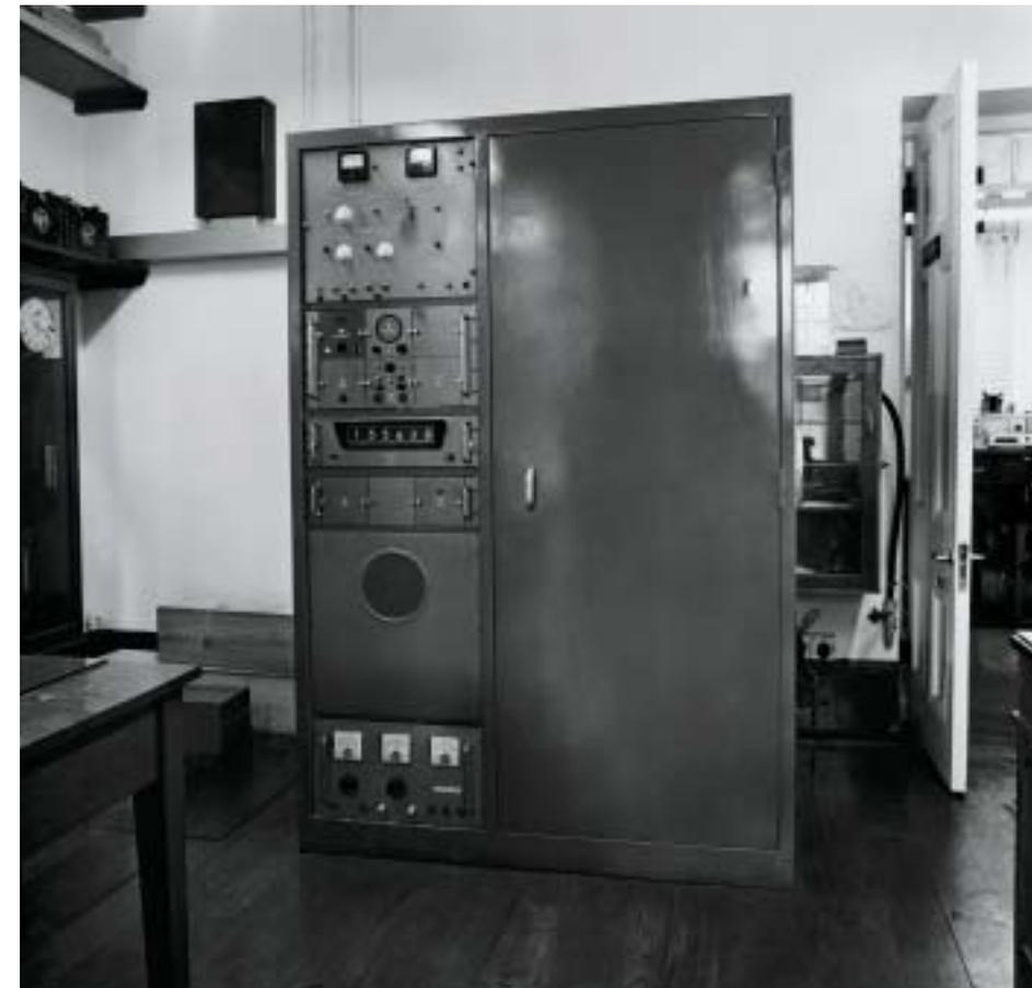
Fig. 3.31 A crystal-controlled timing system of the Observatory installed in 1966. Courtesy Hong Kong SAR Information Services Department
