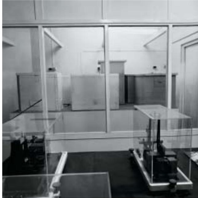
Fig. 3.42 The seismographs are protected at constant temperature and humidity within a double-walled cellar built in 1923. Courtesy Hong Kong SAR Information Services Department
