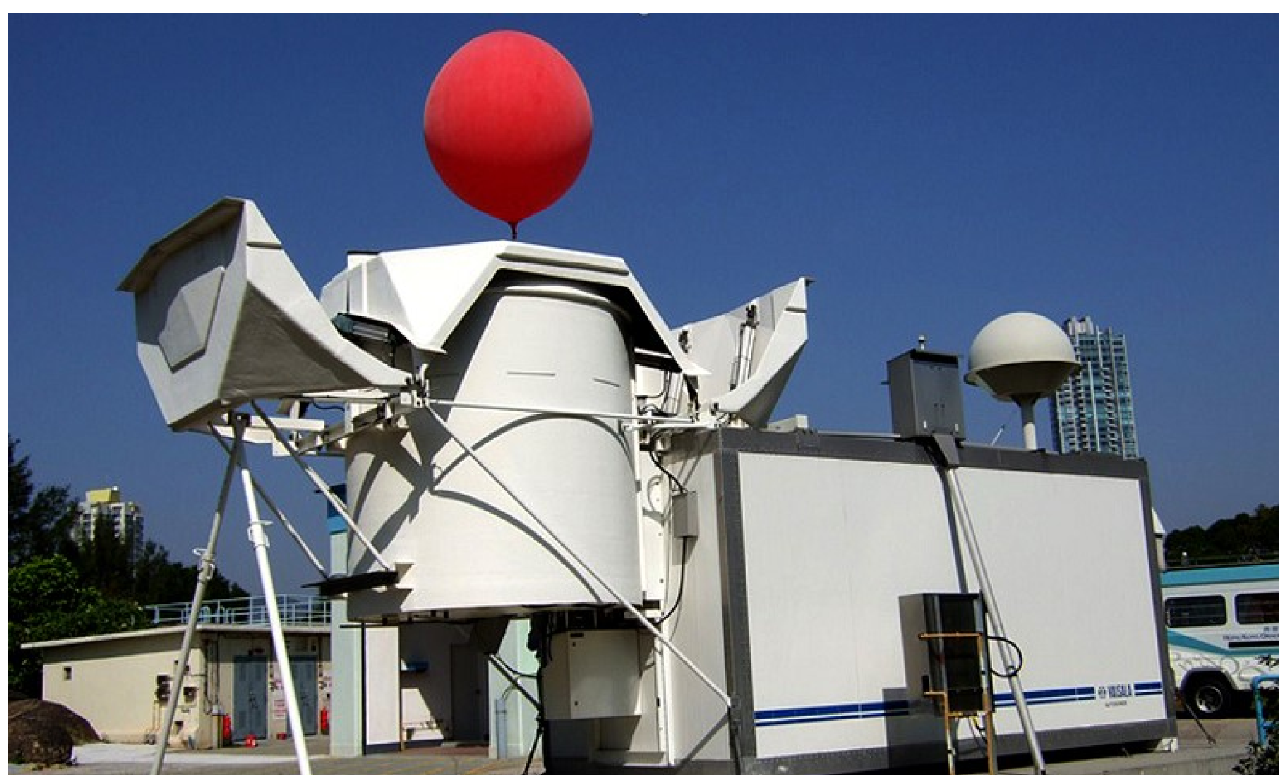
The Automatic Upper Air Sounding System at the upper-air observing station in King's Park
