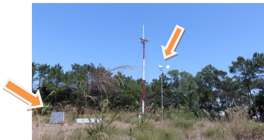
Fig 17: Automatic weather station at Sha Lo Wan using solar and wind power (see arrows).
