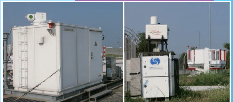
One of the long-range (left) and two of the short-range (right) Doppler LIDARs at HKIA
