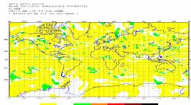
Fig.4c “Mean in-cloud turbulence potential at FL 300”
