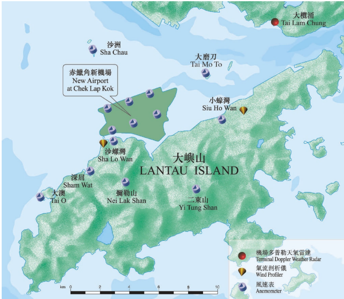
Figure 1. Meteorological Equipment for windshear and turbulence detection at and around Chek Lap Kok
