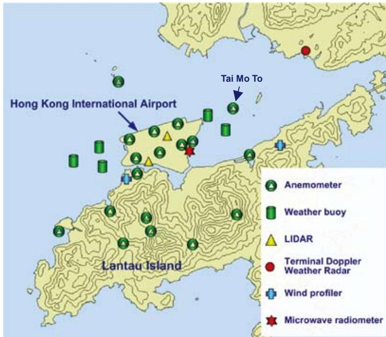
All these data are fed in real time to the Windshear and Turbulence Warning System (WTWS), which is used to automatically generate “up-to-the-minute” **alerts**, when windshear and/or turbulence are detected.
