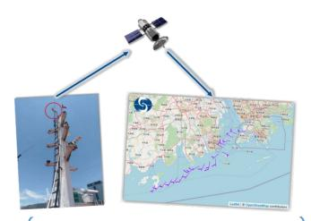
The data measured by anemometers on fishing vessels are transmitted back to the Observatory Headquarters in real-time using satellite communication technology.
