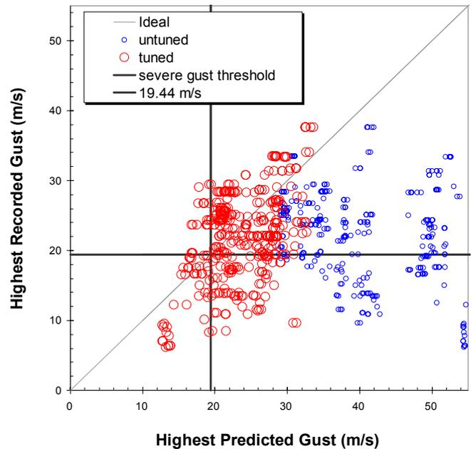
Fig. 5 Scatter plot showing highest recorded gust versus the predicted maximum convective gust in the test data set. Blue and red circles represent respectively predictions before and after tuning.
