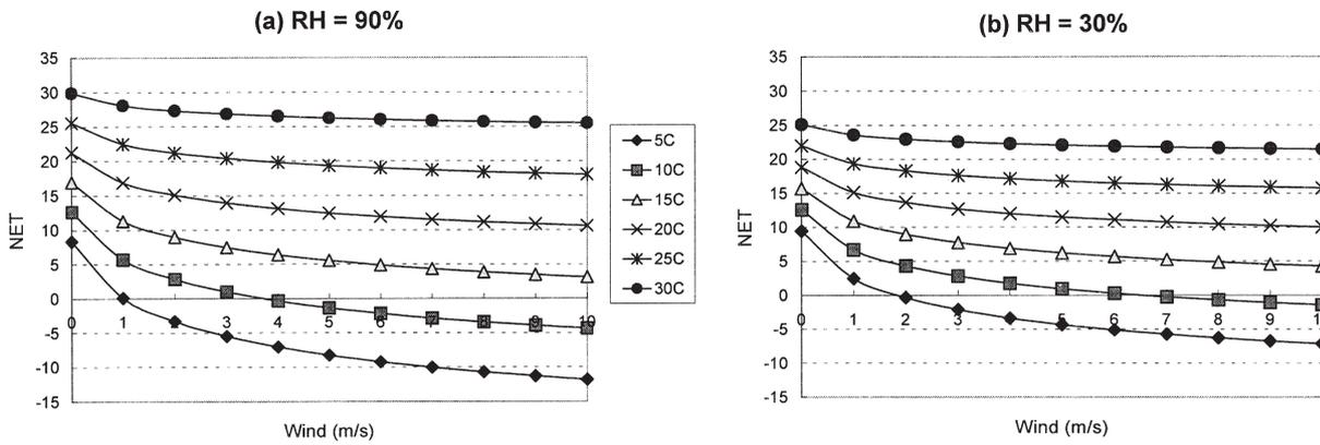
Figure 1. Behaviour of NET as a function of wind and temperature, for (a) wet conditions ( $RH = 90\%$ ) and (b) dry conditions ( $RH = 30\%$ ). Lines with diamond, square, triangle, cross, star, and circle are evaluated at air temperatures of  $5\text{ }^{\circ}\text{C}$ ,  $10\text{ }^{\circ}\text{C}$ ,  $15\text{ }^{\circ}\text{C}$ ,  $20\text{ }^{\circ}\text{C}$ ,  $25\text{ }^{\circ}\text{C}$ , and  $30\text{ }^{\circ}\text{C}$ , respectively.
