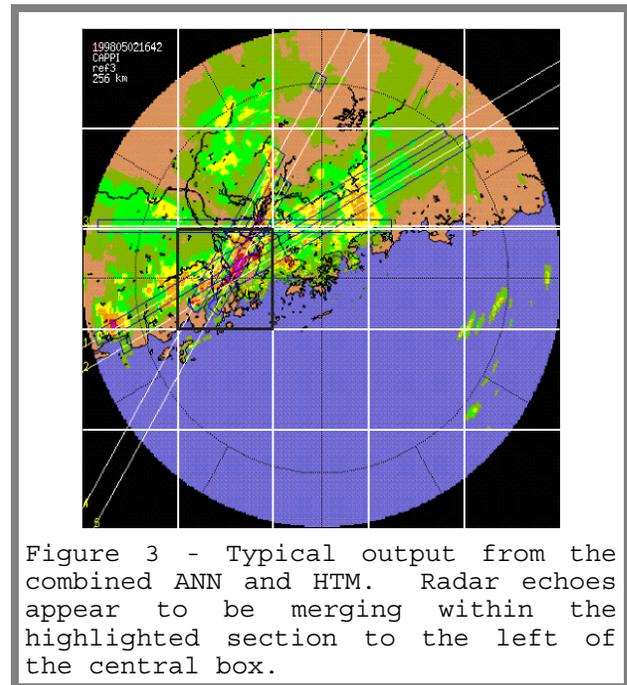
Figure 3 - Typical output from the combined ANN and HTM. Radar echoes appear to be merging within the highlighted section to the left of the central box.
