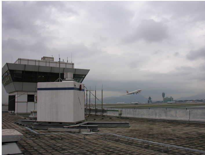
Figure 4 The south runway LIDAR operating at HKIA.
