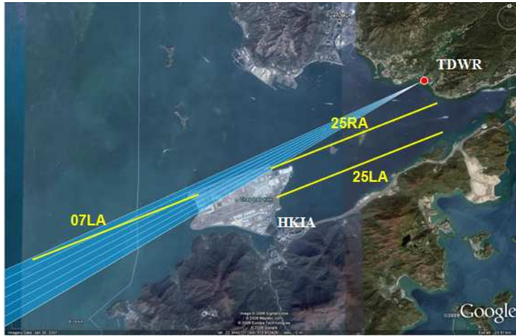
Figure 6 The locations of the TDWR (red dot) and Hong Kong International Airport (HKIA). The blue beams illustrate the radar beams over the runways corridor 07LA of the airport with 1^\circ azimuth interval. Three yellow lines indicate the approach paths and their names are marked.
