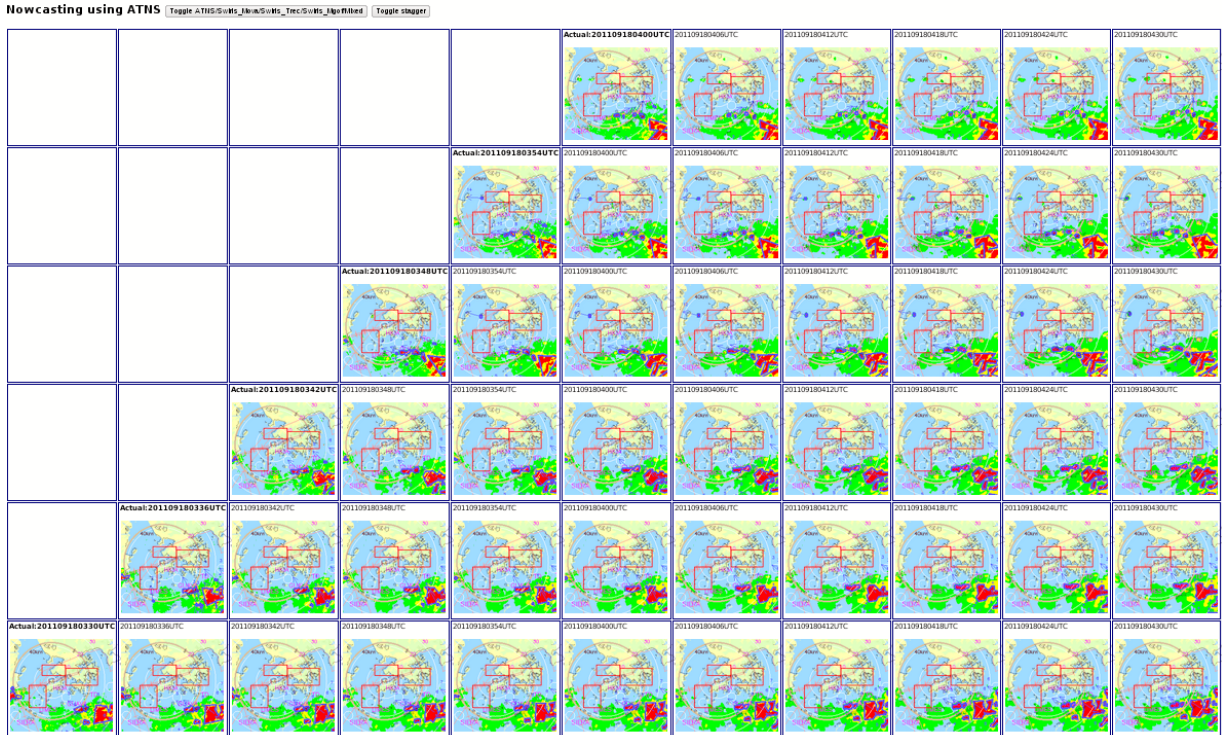
Fig. 6 Screen capture of the combined nowcast viewer in time-staggered display mode with forecasts aligned according to valid times. Each row corresponds to the actual radar observation and the 10 nowcasts from a single run of the selected nowcasting algorithm. The rows are time-ordered with the latest one on top.
