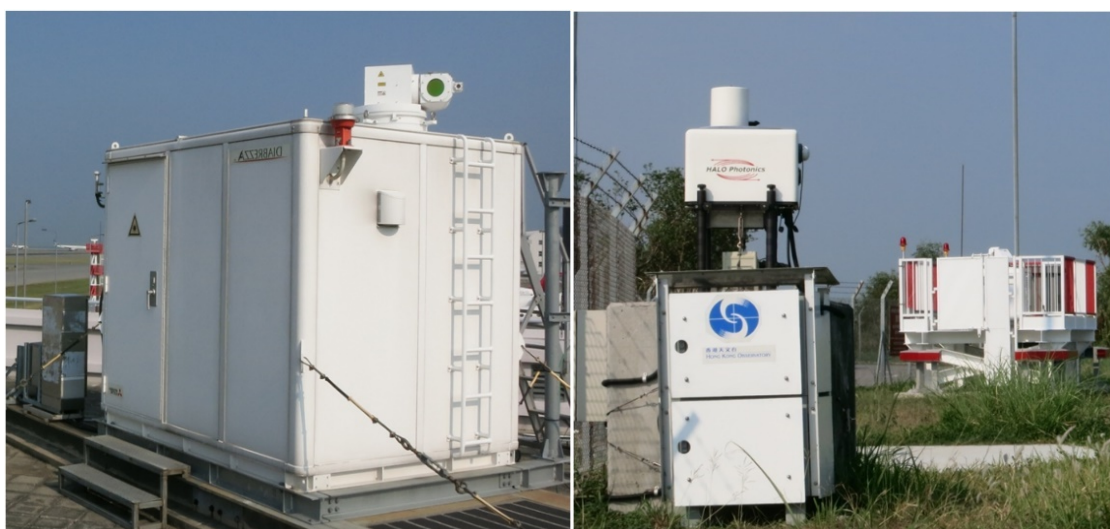
Figure 14 The long-range Doppler LIDAR (left) and short-range Doppler LIDARs (right) at HKIA
