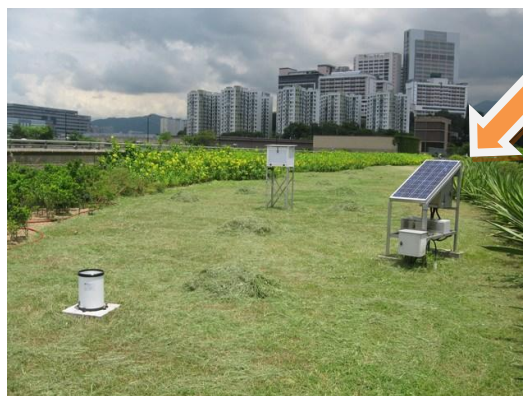
Fig 20: Automatic weather station at Lai Chi Kok Park using solar power (see arrow).
